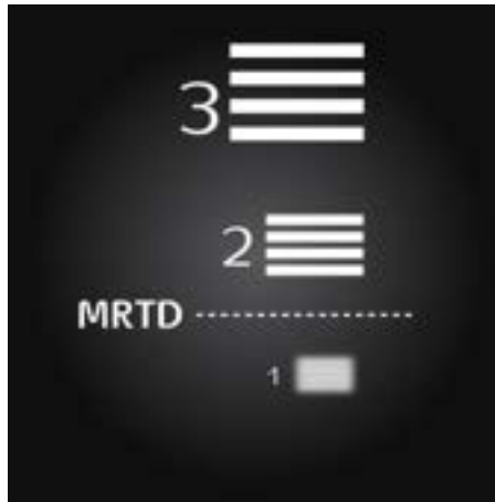
Figure 14 — Illustration of Minimum Resolvable Temperature Difference determination, Opgal company training materials
