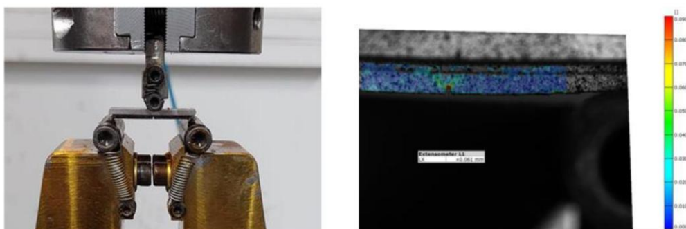
Figure 13 — Fracture toughness test setup for reinforcement and strain at fracture initiation for the reinforcement with a notch of 0.5 mm
