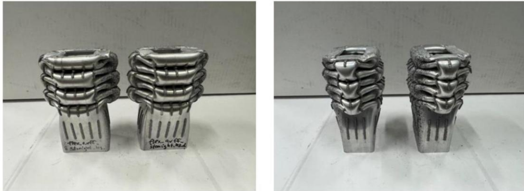
Figure 18 — Crushed crash boxes with straight ribbed reinforcements without cracks and clear folds
