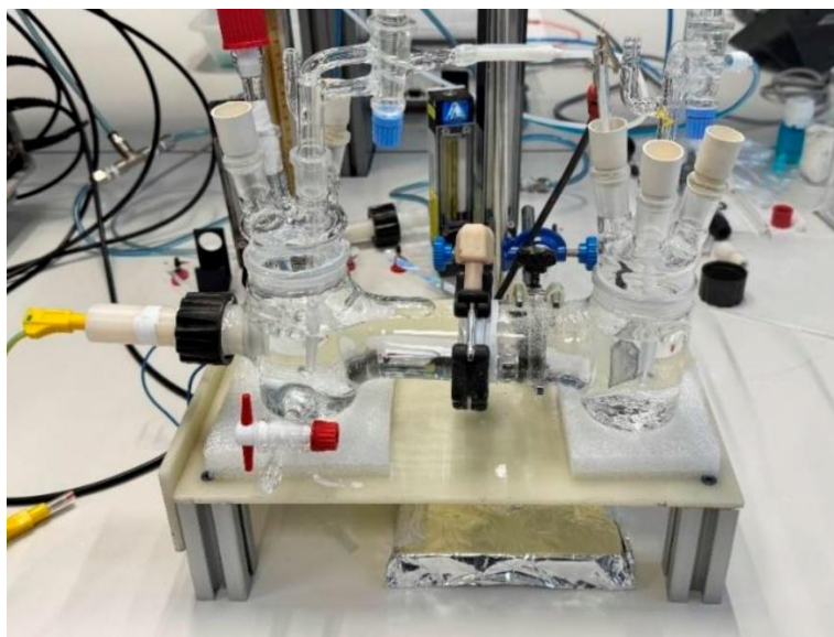
Figure A.1 — The two-compartment electrochemical cell, designed at CIDETEC, employed for performance testing and long-term stability tests
