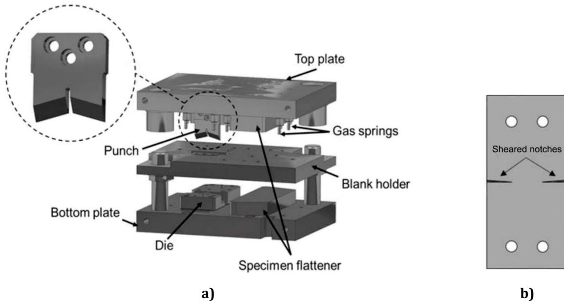
**Figure 13 — a) Tool for introducing sharp notches in sheet metal specimens and detail of the bevelled punch. b) DENT specimen with sheared sharp notches [60]**
