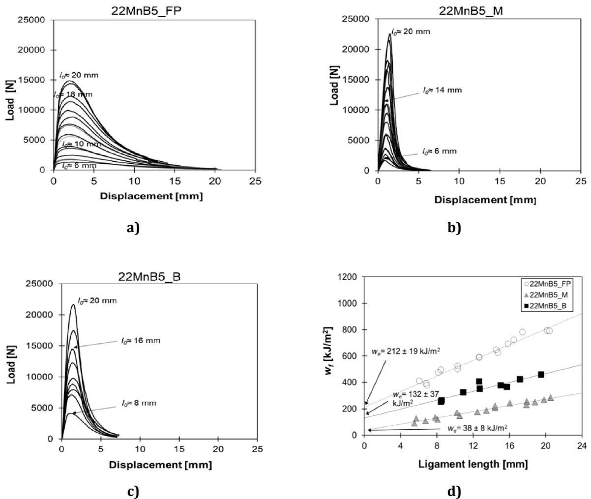
**Figure 9 — Load vs load-line displacement curves from EWF tests with SENB specimens for thick 22MnB5 steel sheets at different conditions: a) As-received state (Ferrite-Pearlite), b) Fully hardened (Martensite), c) Controlled Cooling (Bainite), d)  $w_f$  as a function of the ligament length for the different thick 22MnB2 steel sheets**
