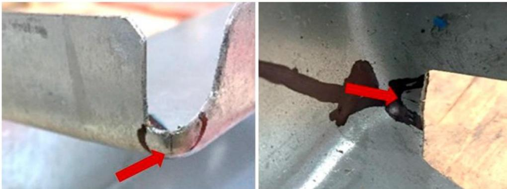
Figure 29 — Edge cracks observed in the component manufactured with DP steel grade [74]
