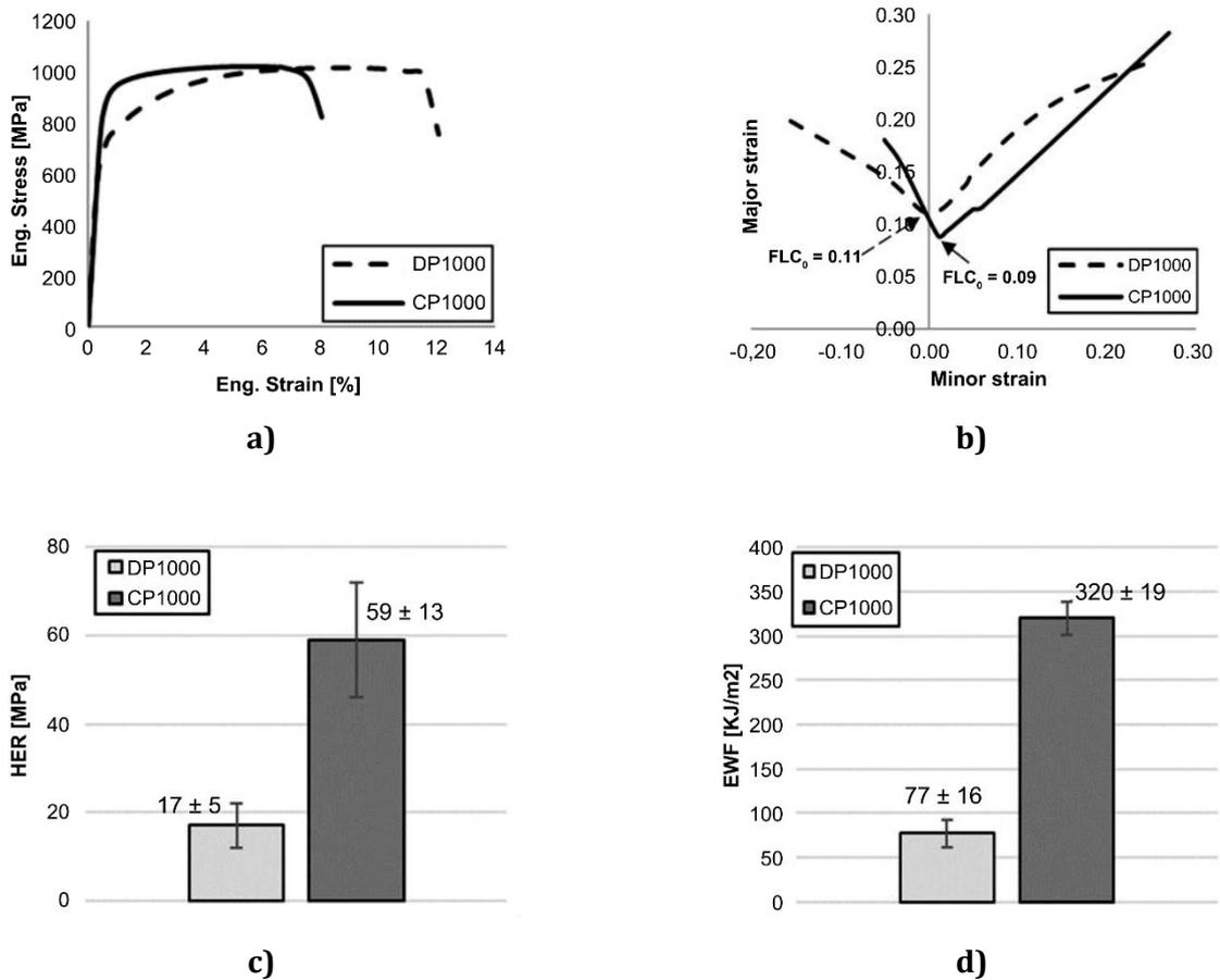
**Figure 30 — Results from mechanical characterizations for the investigated CP and DP grades. a) Engineering stress-strain curves, b) FLCs, c) HER and d) EWF. Image from [74]**
