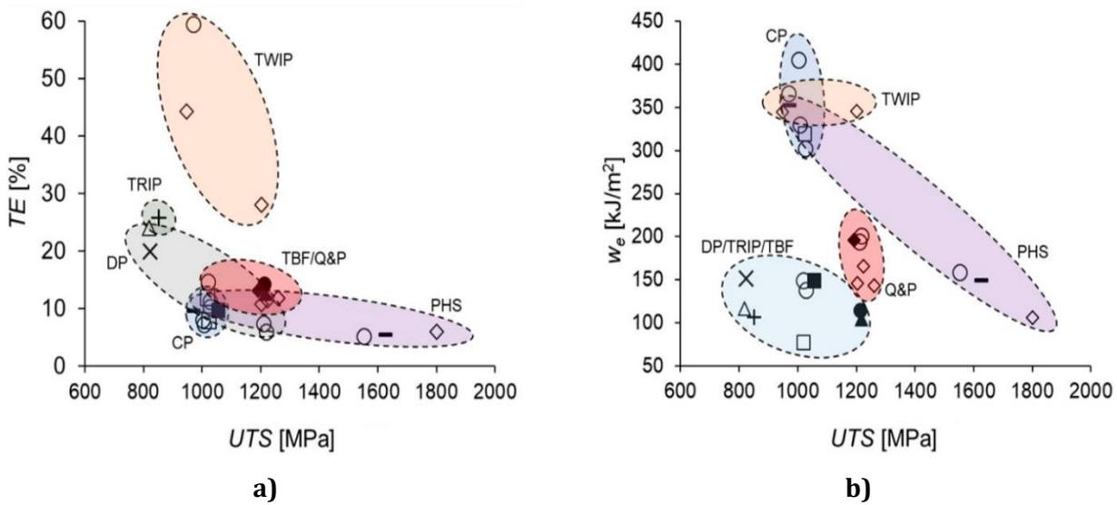
**Figure 25 — a) Conventional classification diagram of AHSS steels (“banana plot”) in terms of UTS and TE. b) Proposed diagram for classification of AHSS according to their strength level (UTS) and fracture resistance ( $w_e$ ) [56]**
