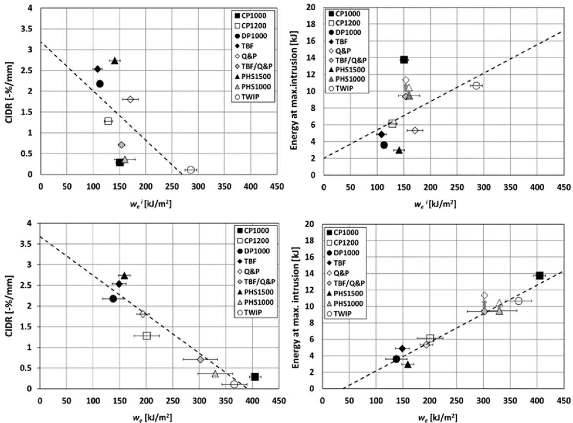
Figure 23 — Crash performance parameters (CIDR in the left and Energy absorbed at maximum intrusion in the right) as a function of fracture toughness parameters ( $w_e^i$  in the top row and  $w_e$  in the bottom row) [71]
