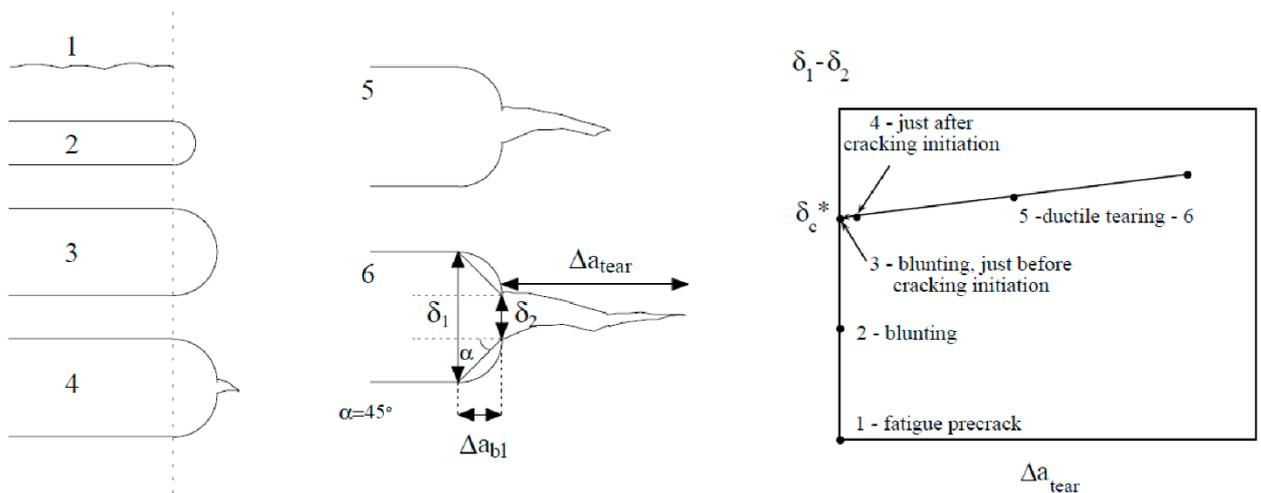
**Figure 11 — Crack blunting before propagation mechanism in a ductile material [59]**
