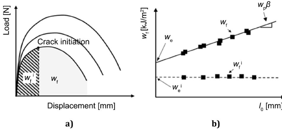
**Figure 7 — Experimental procedure for the determination of the essential work of fracture,  $w_e$  and the specific work for fracture initiation,  $w_e^i$  [10]. a) Determination of the total work of fracture ( $W_f$ ) and total work for fracture initiation ( $W_f^i$ ) from the load-displacement curve, b) specific work of fracture,  $w_f$ , and specific work for fracture initiation,  $w_f^i$ , as a function of the ligament length,  $l_0$**
