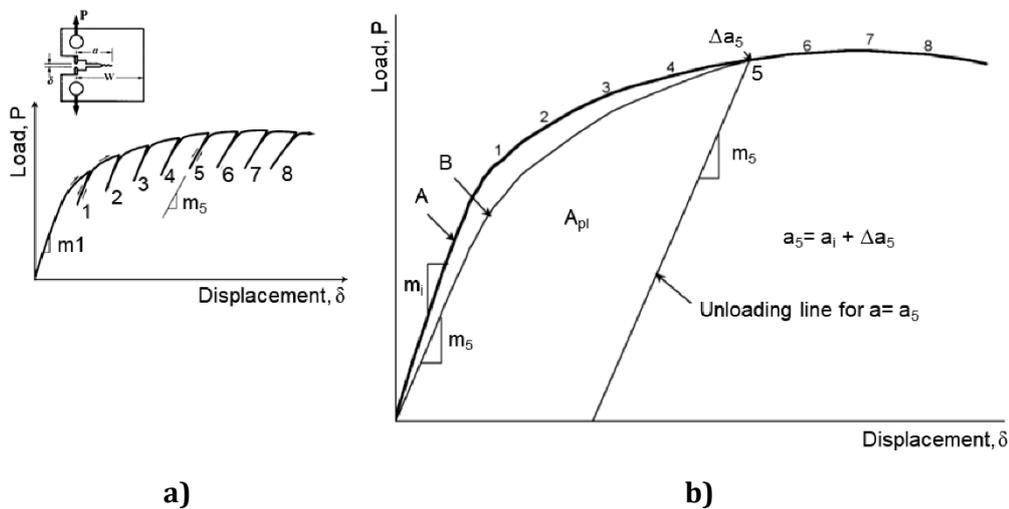
**Figure 2 — a)  $J$  determination through partial unloading cycles following the compliance method; b) Plastic area,  $A_{pl}$ , to calculate the  $J$ -integral. The curve A represents the actual load-displacement curve of the growing crack. The curve B corresponds to the hypothetical load-displacement curve for a stationary crack with length  $a_5$  [11]**
