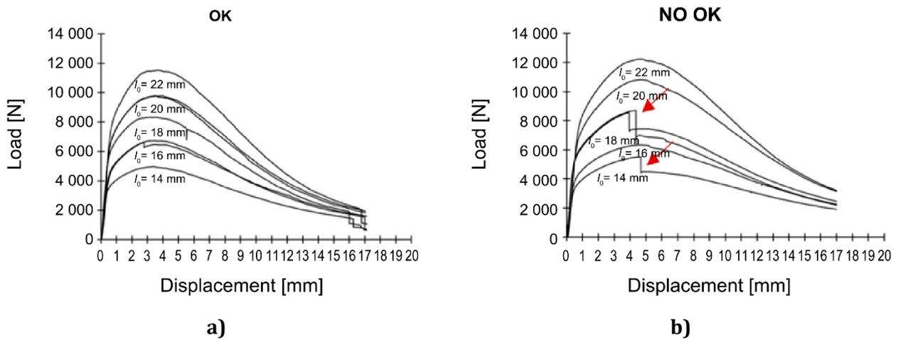
Figure 28 — Load-displacement curves obtained for two steel batches: OK (a) and NO OK (b)
