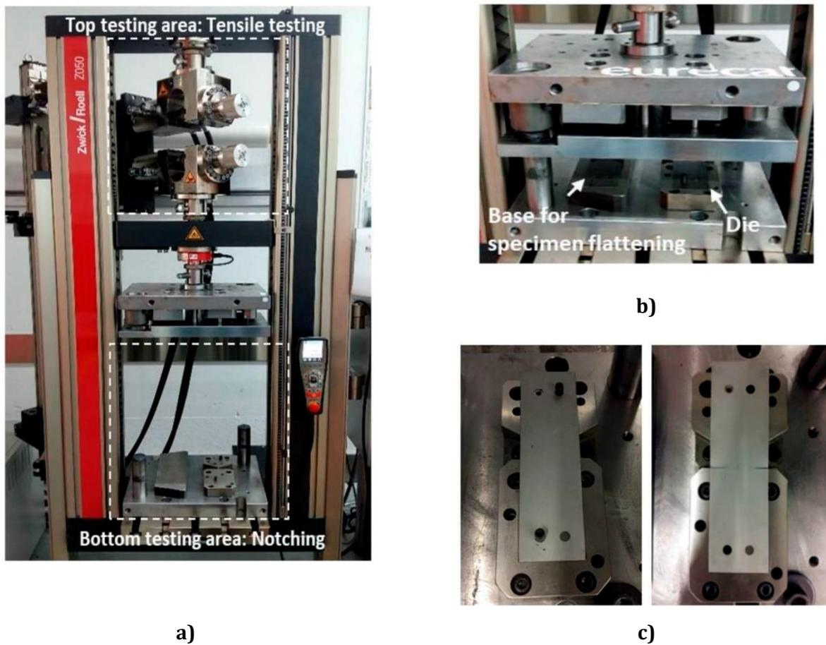
Figure 14 — Images of the experimental setup for the notching process. a) Setup of the tool in the testing machine. b) Detail of the cutting tool. c) Specimen before (left) and after (right) the notching process [60]
