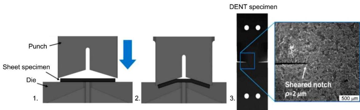
Figure 15 — Schematic representation of the experimental procedure for the preparation of sheared notches in sheet specimens [60]
