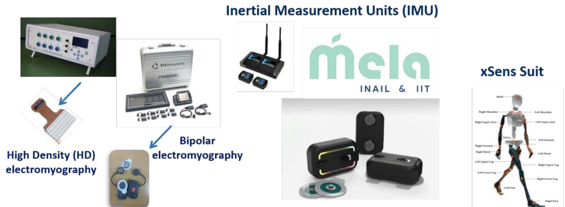
Figure 1. Example of wireless wearable sensors: high density (HD) and bipolar sEMG sensors and IMUS.
