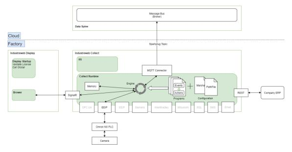
Figure A.6 — Factory Connector Architecture
