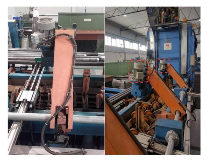
Figure A.13 — Installed sensor on polishing machine
