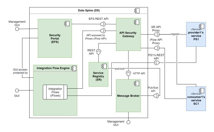
Figure 12 — Synchronous services' integration through the Data Spine.
