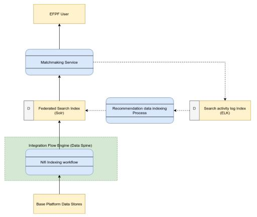
Figure 21 — Data Flow in Matchmaking Components
