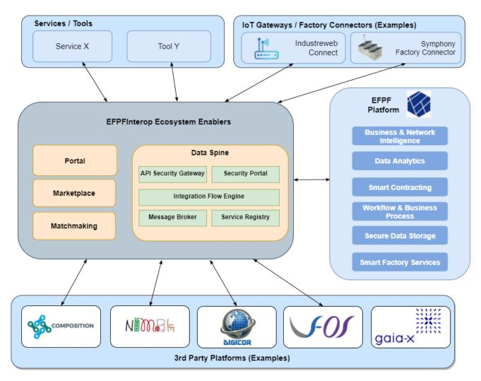
Figure 4 — EFPFInterop Ecosystem Enablers with components
