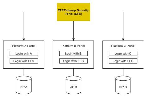
Figure 6 - An illustration of 'Login with EFS' option on the platforms' Web portals
