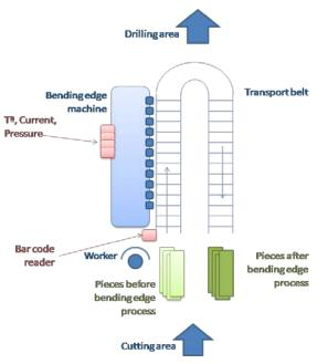
Figure A.3 — Diagram of the preliminary placement of the devices
