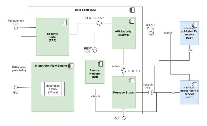
Figure 14 — Asynchronous services' integration through Data Spine.
