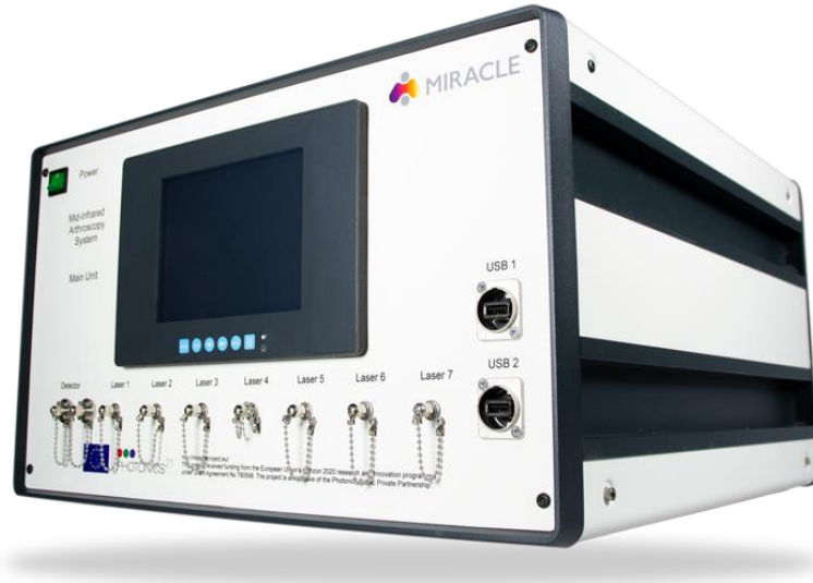
Figure 3: MIRACLE 19" unit containing 7 lasers as depicted in figure 2 and one detector
