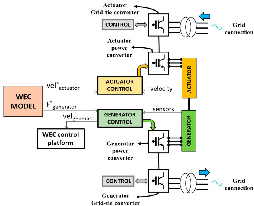
Figure A.8 — HIL testing scheme used for PTO validation
