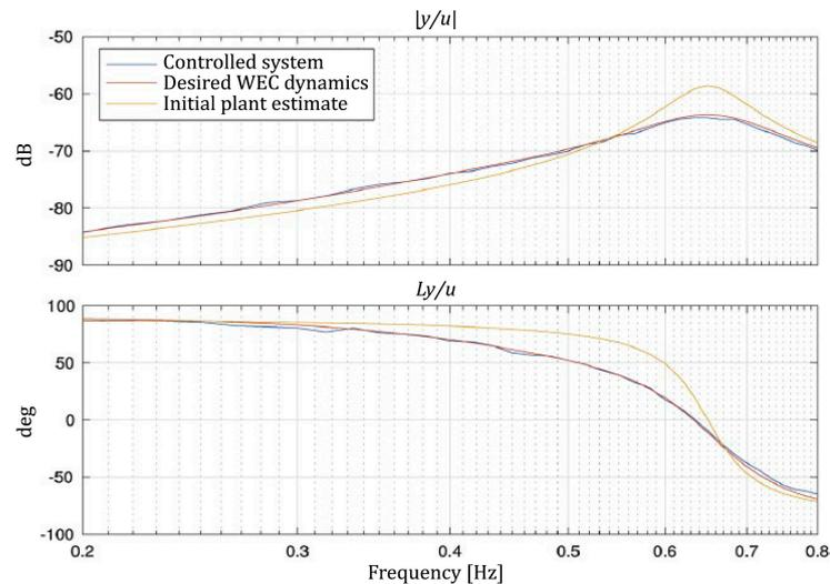
**Figure A.14 — Frequency response function (in terms of magnitude and phase) for bench test system dynamics matching**
