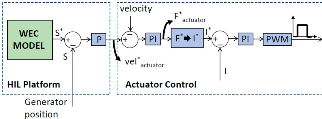
Figure A.7 — Interaction between the HIL control and the actuator control
