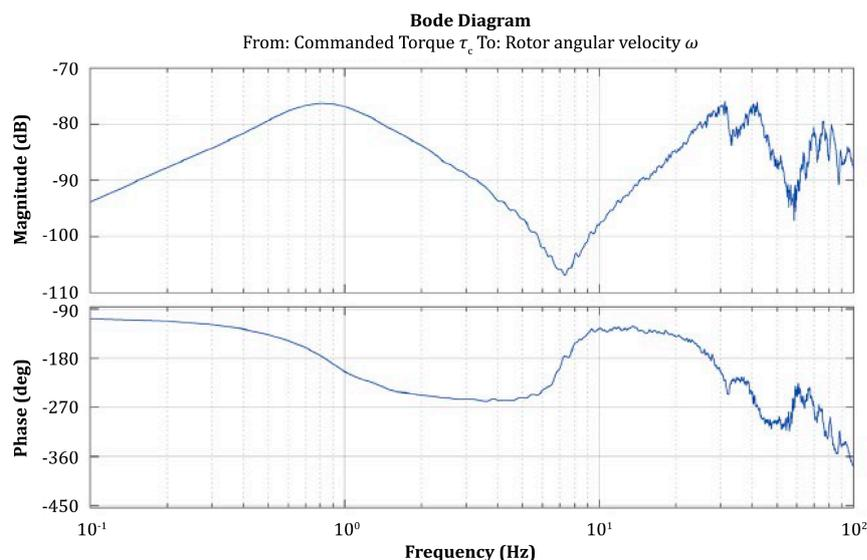
Figure A.12 — Estimated FRF between measured torque and rotational velocity (taken from [1])
