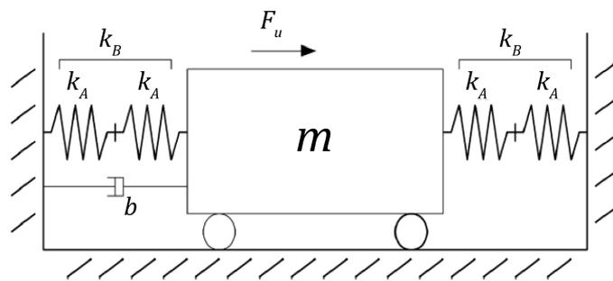
**Figure A.10 — WEC spring-mass-damper system diagram (taken from [1])**
