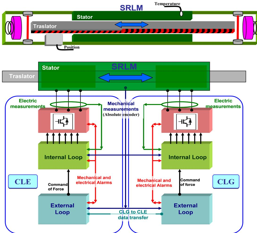
**Figure A.6 — Electric schema for testing the machine using half of the machine as actuator and the other as generator**
