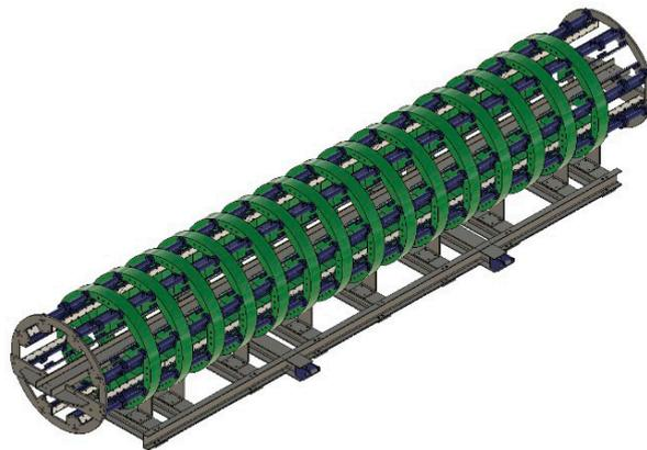
Figure A.1 — 3D view of the linear generator
