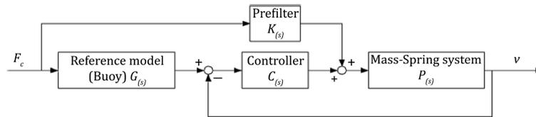
Figure A.13 — Block diagram of control system for dynamics matching (taken from [1])
