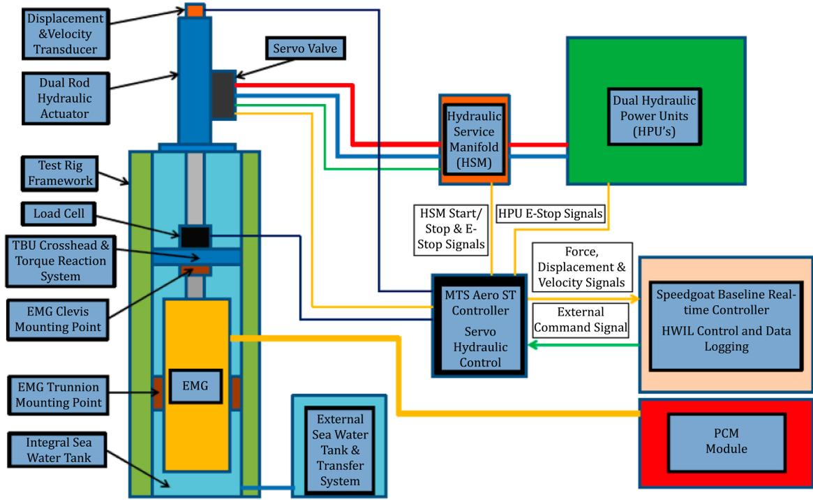
Figure A.15 — Diagram of hardware test bench unit architecture (taken from the information from UMBRA)
