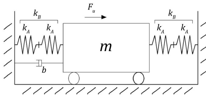
**Figure A.10 — WEC spring-mass-damper system diagram (taken from [1])**
