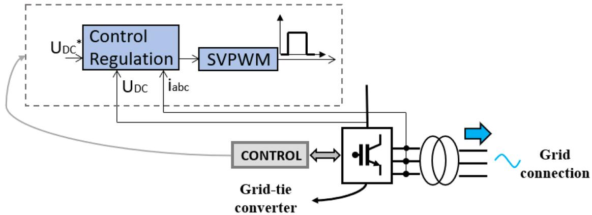
Figure A.5 — Grid-tie converter control
