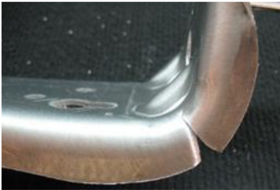
Figure 31 — Edge fracture in a cold-formed automotive component manufactured with a series 5xxx aluminium alloy
