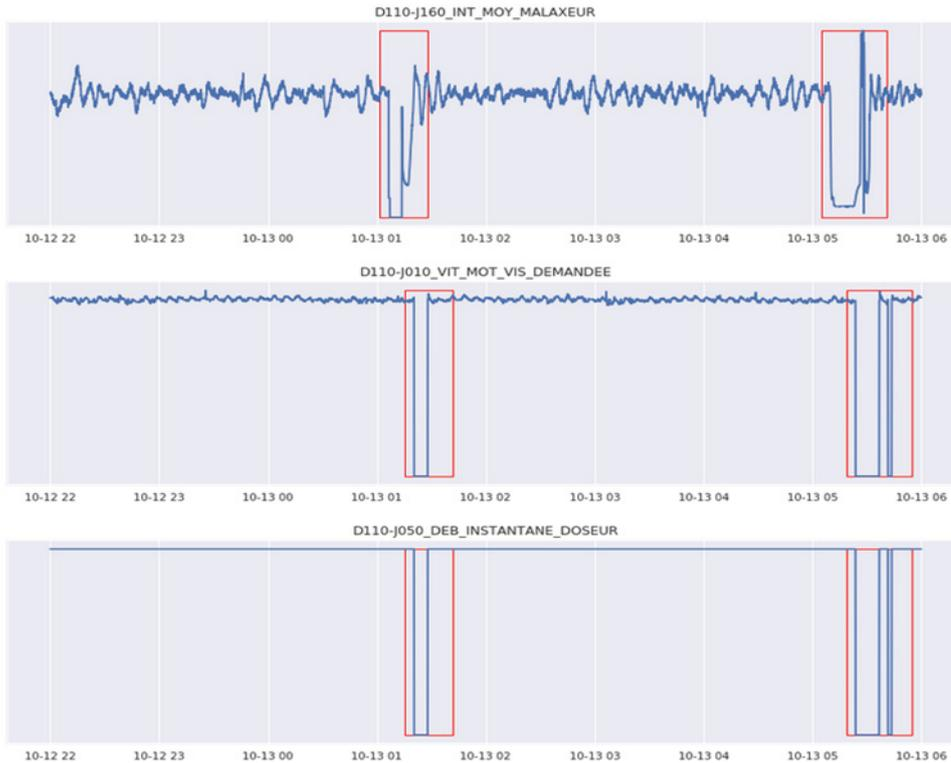
**Figure 2 — Example of signals used for identifying paste plant stops – The periods in red are identified as stops**
