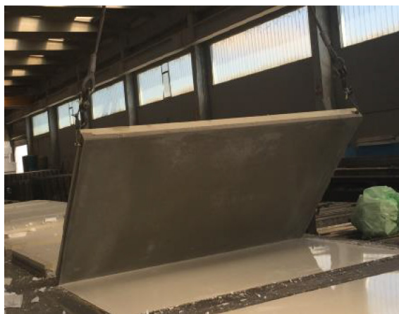
Figure 23 — The panel being demoulded and put in vertical position with the overhead crane
