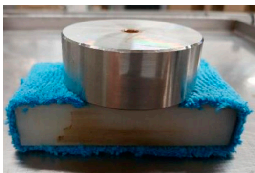
Figure 3 — Cleaning cloth fixed to the support.
