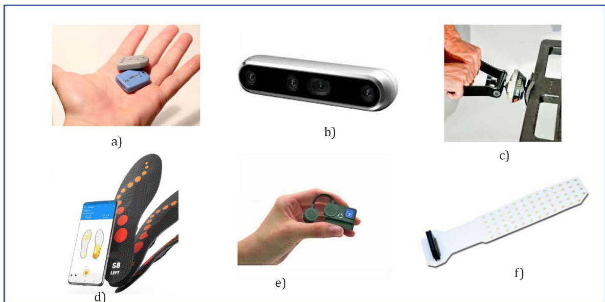
Figure 1 — IMUs a), 3D depth cameras b), Force measuring devices c), sensorized insoles d), bipolar e) and HDsEMG f)
