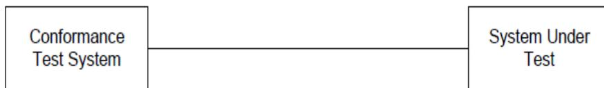
**Figure 4 — The principle of conformance testing**
