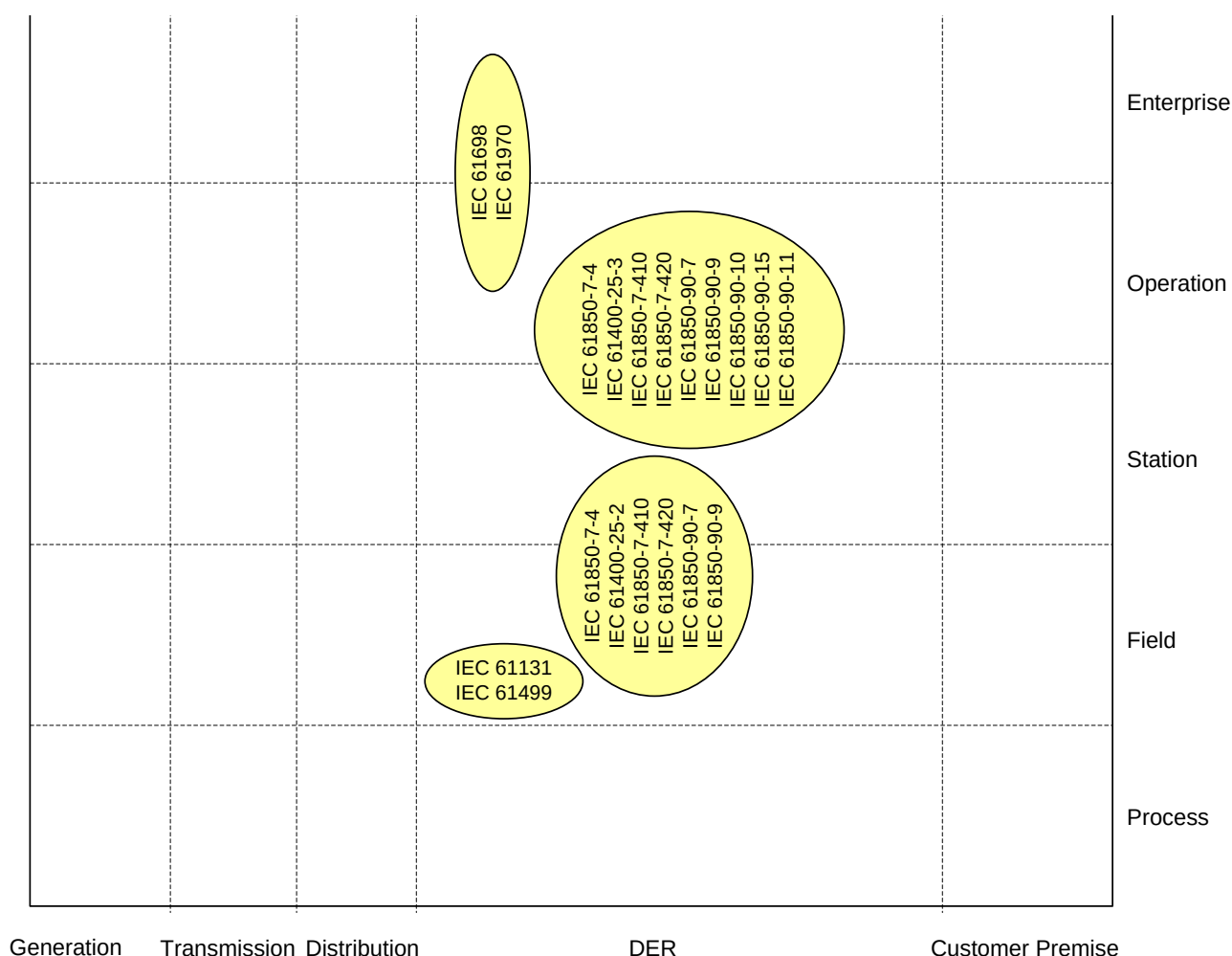
Figure 32 - DER operation system - Information layer
