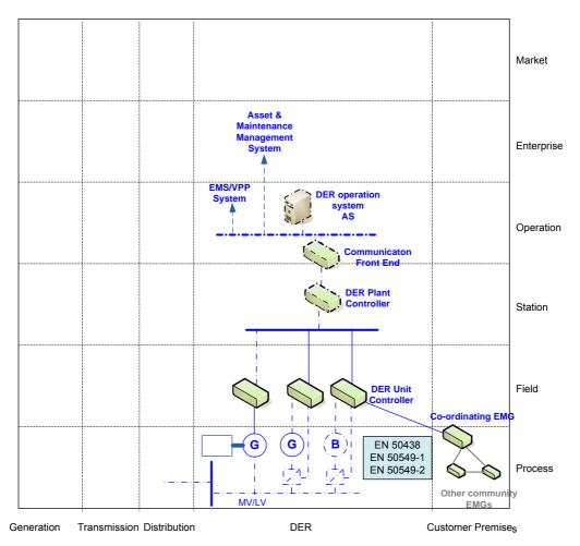
Figure A-4 : Mapping of WGSP-2137 to the SGAM Component Layer
