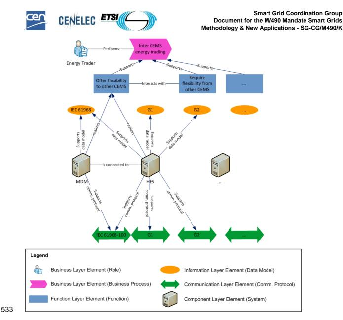
534 **Figure 4: Example of interrelationships between concepts on different levels in an SGAM model** (for details refer to Appendix A)
