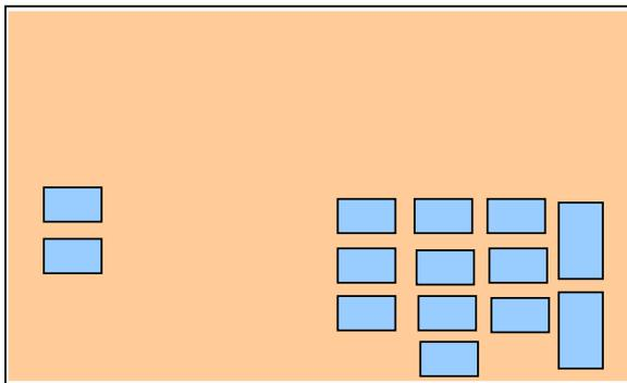
**Example 2** – this shows a monitor with two Touch Frames and 14 Touch Keys. The space within the Touch Frames not defined by a Touch Key are inactive (do not respond to touch). All areas outside a Touch Frame operate in Mouse mode. This example shows two Mouse mode "keys". e.g. Windows "Button", HTML "BUTTON" or a custom control. Other touches in Mouse mode are normally dealt with by the application event engine. However, this can be restricted – see example 3.
