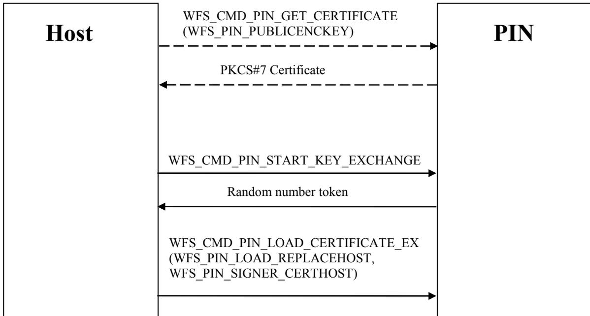
NB: Dotted lines represent commands that are only required if the PIN device encryption certificate has not been previously stored by the host.
