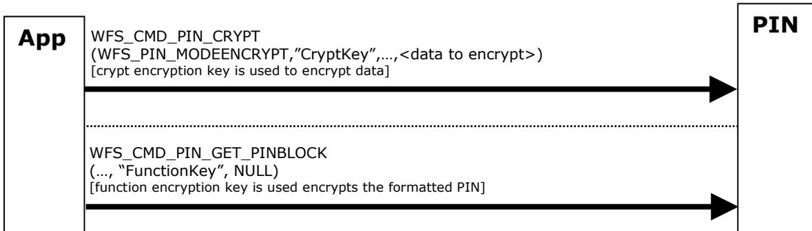
Master key restriction disallows loading of derived keys with different usage:
