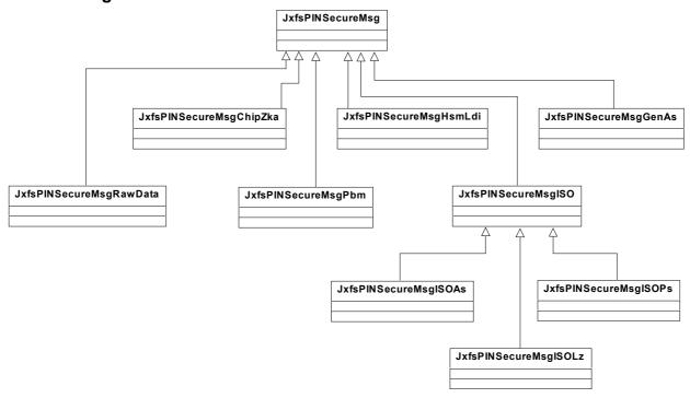
All message classes are derived from the global abstract JxfsPINSecureMsg class. The access to the binary message data is done via the synchronized getMessageData() and setMessageData() methods. If the message data will be modified, the whole message has to be set.
